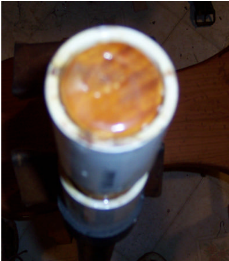
PVC epoxied over end of rod
